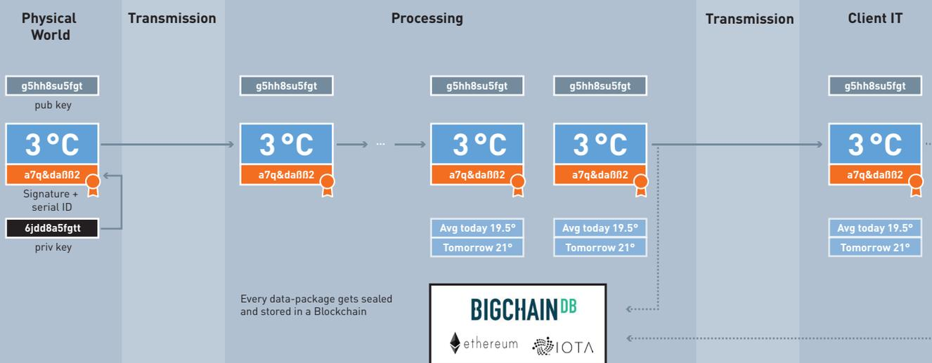
The UBIRCH solution attaches a cryptographic signature on every data-package from an IoT device
