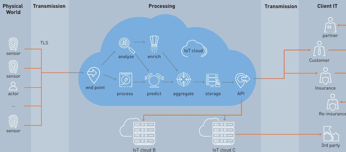
Securing the tunnel does not work well in more complex data-ecosystems
