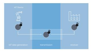
Conventional TLS encryption only protects IoT devices and transmission paths. The data itself can be hacked and tampered with.
