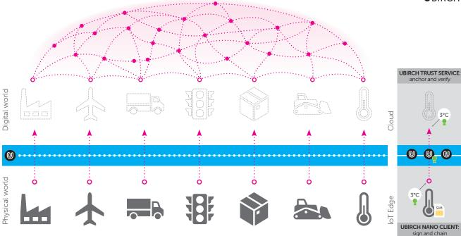
**The physical world with its digital shadow** – The ubirch nano client software is running on the edge device, for example on 1NCE SIM cards, signing and chaining data at the source of data creation. The cloud-based ubirch trust service is anchoring the trusted data into the blockchain and offering simple REST-based services for verifying received data regarding its authenticity and integrity against the blockchain.
